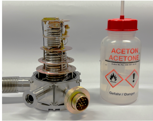
FIGURE: Photograph of the sionludi XS , an ultra-compact dilution refrigerator. It features standard cryogenic components, including three precooling stages at 100 K, 20 K, and 4 K, as well as a base stage at 70 mK.
